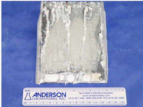
HDG G40 + CG-AG Overbend (Tool Defects)
